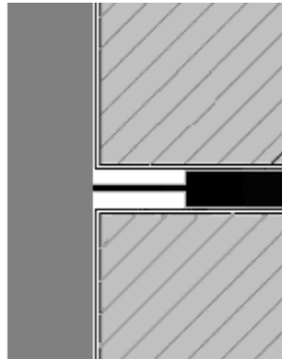
Camera face on door exterior 3/4" Dia. x 1/16" D
